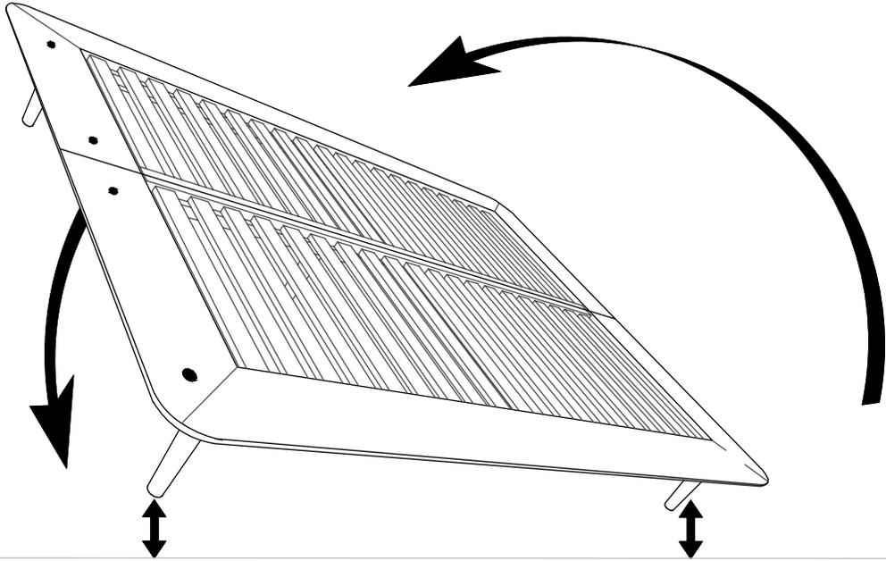
6. Attach headboard to frame using flat washer and short M8 bolt, as shown. Tighten bolts evenly with 5mm Allen wrench.
