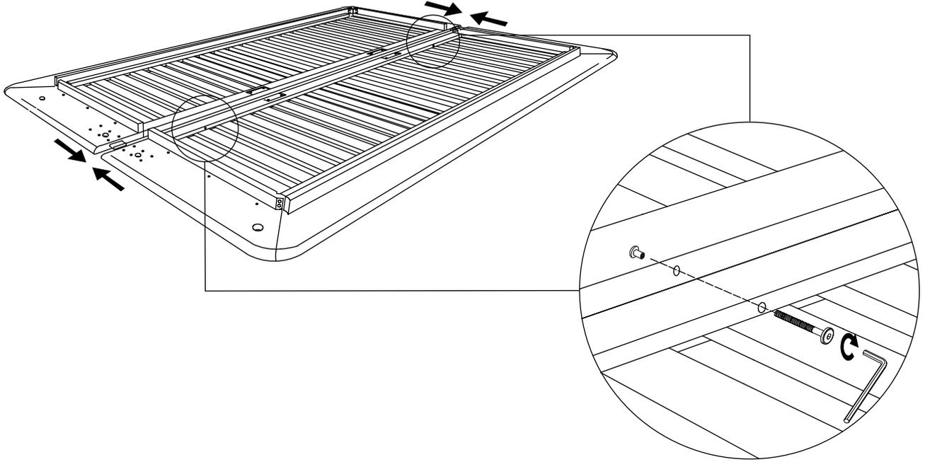
2. Attach either leg assembly to bed frame with six long M6 bolts, as shown, threading all loosely but waiting to tighten fully until next step. Repeat with other leg assembly.
