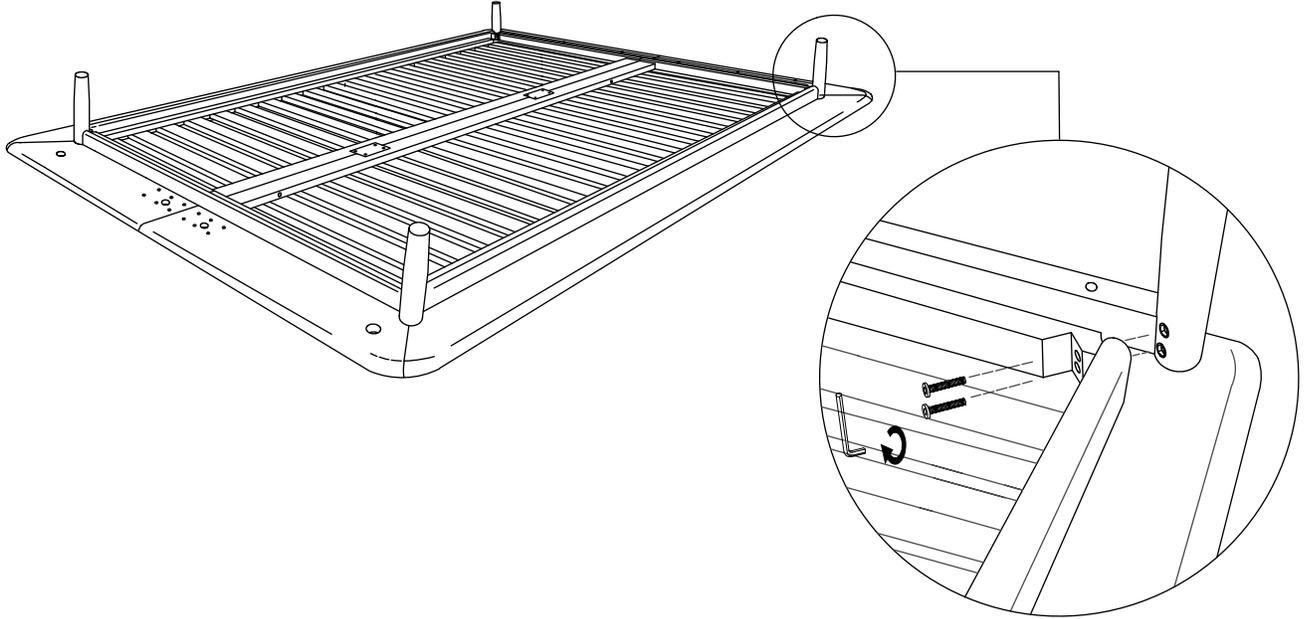
4. Attach either center leg to frame using four short M6 bolts, threading all loosely at first then returning to tighten fully with 4mm Allen wrench. Repeat with other leg. Install base plate on either end of bed with 12 short M6 bolts, threading all loosely at first then returning to tighten fully with 4mm Allen wrench. Repeat with other plate.
